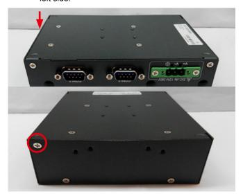
Step 4 Remove one FHS-M3x4 screw (circled in red) on the right side.
