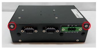
Step 3 Remove one FHS-M3x4 screw (circled in red) on the left side.
