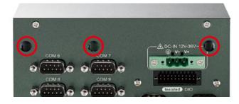
Step 3 Put antenna cable connector into the hole on rear panel.
