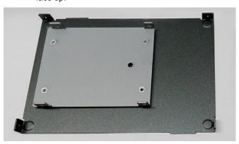
Step 3 Make sure the directions of SPC-3000's lower cover and SSD/HDD match.
