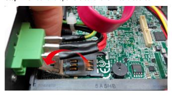
Step 2 Install SIM card into SIM card socket.
