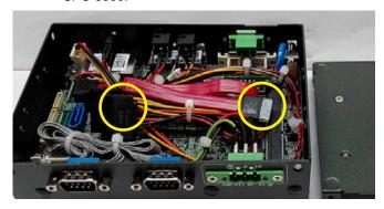
Step 6 Plug in SATA data cable and SATA power cable to SSĎ/ HDD.
