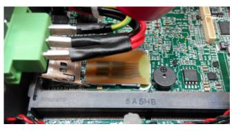
Step 3 Close and lock the cover of SIM card socket.
