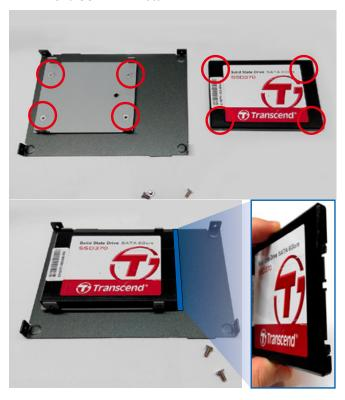
Step 4 Fasten the four KH-M3x6 screws.
