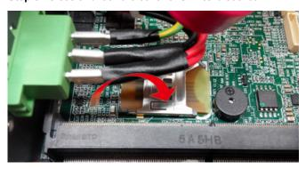
1.6 Installing SSD/ HDD
