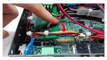
Step 2 Make sure the RAM module is well-locked by the memory slot.
